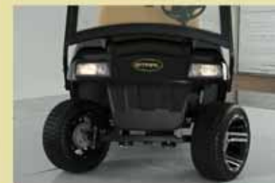
Rack and pinion steering; solid front bumper
