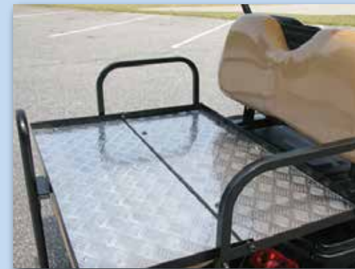
Flip seat with aluminum plate
