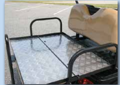
Flip seat with aluminum plate
